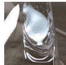
A clear visor molten by radiant heat
